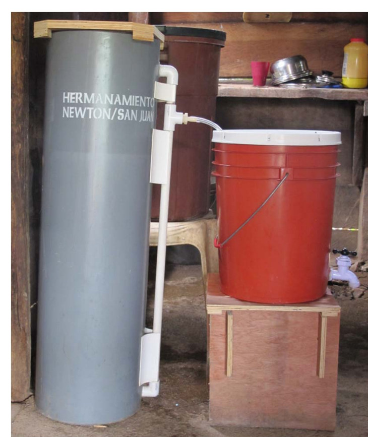
Figure 2: Locally-built PVC (Large) and 5-gallon Bucket (Small) Casing BSFs (Photos by Anna Murray)
