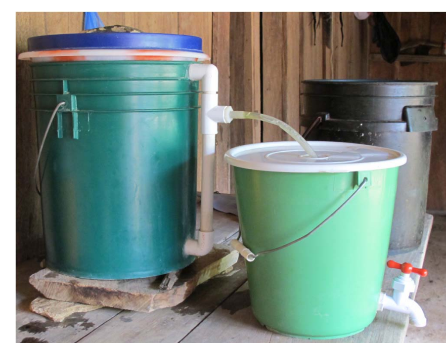
Figure 2: Locally-built PVC (Large) and 5-gallon Bucket (Small) Casing BSFs (Photos by Anna Murray)
